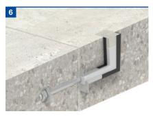
After 24 hours the void former can be filled with cementitious material, level with the top of the slab, to complete the installation.
