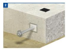
Pour the concrete, and when of sufficient strength, strike the formwork. Puncture the label to reveal the cylindrical sleeve only and insert the dowel until it is approximately 20mm from the back of the void former.
