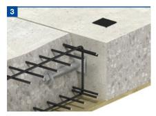
Fix the local reinforcement around the dowel component and pour the concrete.
