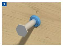
Nail the threaded anchor to the formwork so the dowel will be central in the adjoining slab or within 150mm of the top of slabs over 300mm. Fix the local reinforcement as specified on engineer's drawings and cast the concrete.
