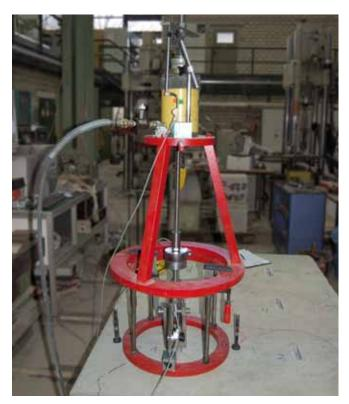
Test setup; pull-out test
