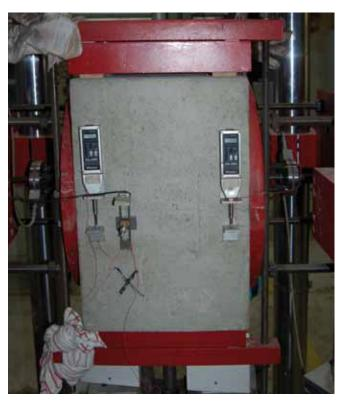
Test setup for cyclic load test
