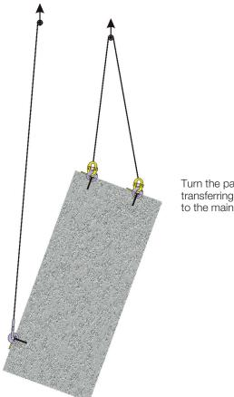
Turn the panel by transferring the load to the main hoist.
