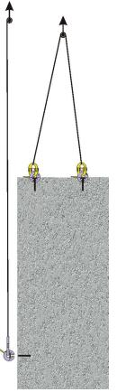
Remove the spin-up clutch. Hoist the panel into position and disconnect the top lift clutches, preferably with the aid of an elevated work platform.
