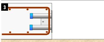
When the concrete has achieved sufficient strength, strike shuttering and peel off or puncture the label
