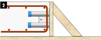
2 Fix the local reinforcement around the sleeve and pour the
