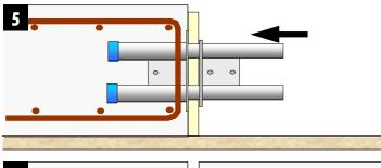
Push the dowel component through the filler until it is fully located in the sleeve
