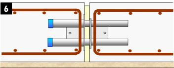
Fix the local reinforcement around the sleeve and pour the
