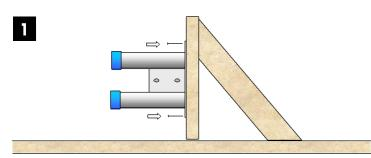
Nail sleeve to formwork. Do not remove sticky label, this prevents ingress of concrete into the sleeve
