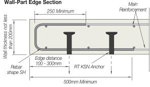
Reinforcement: Minimum edge reinforcement, 12mm diameter Grade 500E The main reinforcement can be detailed to incorporate the above shape noted as rebar SH
