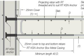
Slab Reinforcement lapped to projecting rebars. Provide bottom bar, Mark (1) with U shaped end
