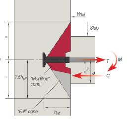
Fig 2. Idealised modified concrete failure. Single line of Anchors is shown.
