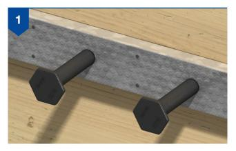
Nail the metal casing to the formwork. The wall reinforcement is installed to which the anchors are tied. The concrete is cast and once it reaches sufficient strength, the formwork is removed to reveal the steel cover.
