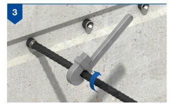
The RT parallel threaded reinforcing bar is rotated into the RT KSN Anchor and tightened using a wrench. No more than 2mm of thread should be left exposed on the bar. Fix the slab reinforcement and pour the concrete to complete the installation.
