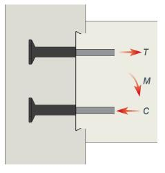
Load condition: Anchor: Method of fixture: Anchor effective embedment: Anchor spacing: Concrete: Slab depth: Wall depth: Anchor reinforcement location: Cover: Moment connection RT KSN20S x 150mm long RT KSNBOX casing 36mm deep 180mm 250mm 32MPa 250mm 300mm Top and bottom of slab 25mm to top main steel
