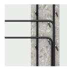
Traditional slab-to-wall construction method. Projecting reinforcing bars and congestion in the wall.
