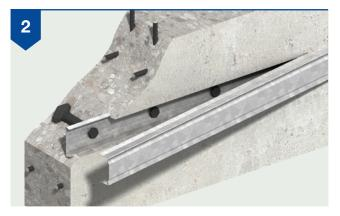
When a connection is required, the cover is removed and the bolts which held the Anchors to the casing prior to installation are removed to reveal the threads.
