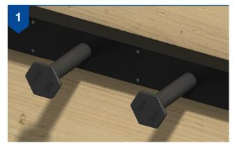
RT KSN Anchors are inserted into the Ancon RT KSN Anchor Block. The unit is then nailed to the formwork. The wall reinforcement is installed to which the anchors are tied. The concrete is cast and once it reaches sufficient strength, the formwork is removed.
