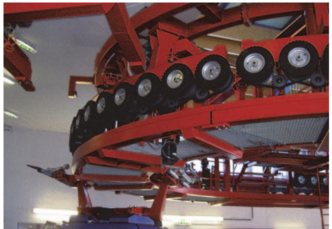
Fixing of the drive unit for a ski lift
