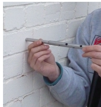
2. Fit the appropriate sized Load Test Key (LTK) at least 50mm (normally one full turn) over the end of the tie. Remove the cross pin, if fitted.
