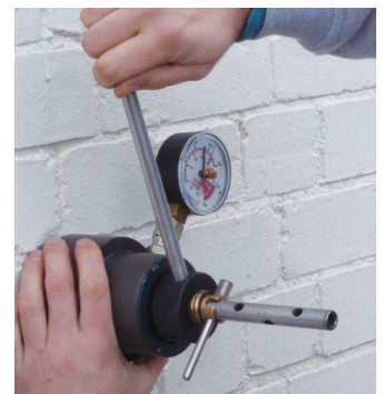
5. Turn the Tommy bar slowly until the proof or maximum load is achieved. DO NOT enter the red zone and DO NOT OVERLOAD .
