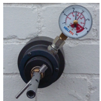
6. Note the reading and then release the tension on the tested wall tie.
