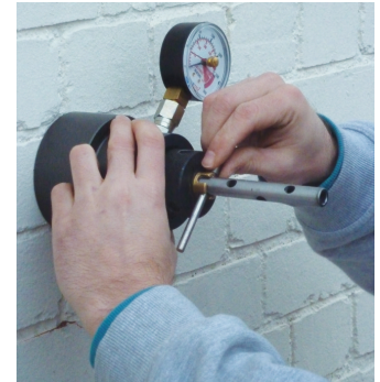
4. Place the cross pin through the LTK and take up the slack on the central nut.
