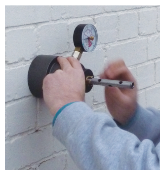
3. Slide the Load Test Unit (LTU) over the LTK and replace the cross pin, engaging it in the castellation on the top of the centre stud.
